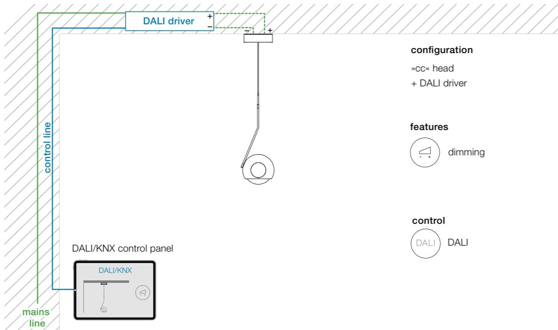
> mains line and DALI control line can be joined in a 5-pol. cable
